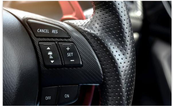
Adaptive cruise control (ACC) is an available cruise control system for road vehicles that automatically adjusts the vehicle speed to maintain a safe distance from vehicles ahead. ACC systems allow your car to maintain a desired speed until it encounters slower-moving traffic. ACC will accelerate or brake to maintain a set distance from the car ahead.
